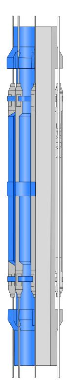
The **PetroQuip Control Line Filter** filters hydraulic fluid in control lines before entering downhole tools to at least 10 microns, safeguarding equipment with NAS6 fluid. Each filter has a built-in contingency feature to bypass the screen and sump area if the filter is plugged, ensuring fluid will always pass through and operate tools below.
