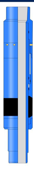
The **PetroQuip Open Hole Packer** is a single element open hole packer that provides high-performance zone isolation, during stimulation, and provides water and gas isolation. The hydraulically set packer combines the sealing strength of a mechanical element with the setting force of a dual-piston cylinder and mechanical body-lock system.
