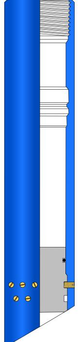
The PetroQuip Pump-Out Wireline Entry Guide (WLEG) provides a means of isolating the wellbore during completion installations. The Pump-Out portion of the WLEG can be manufactured from a glass disk or dissolvable material depending on the application. Unlike other Pump-out subs, the PetroQuip Pump-Out WLEG has a profile machined above the Pump-Out section to allow future isolation operations.
