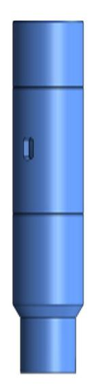
**PetroQuip's SandStorm-S** separates sand and other solids from the produced fluid before it enters the Sucker Rod Pump (SRP). The vortex created inside the tool pushes sand and solids down into a sump or tail pipe below. The unique design has no internal fins or baffles which creates longer tool life. The geometry design has been optimized for the lower flow rate of an SRP.
