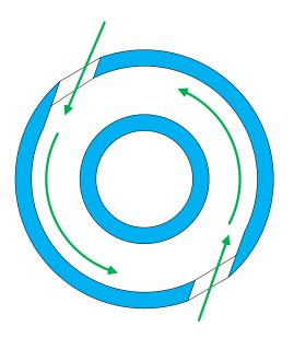
Flow enters through a port tangentially here. The way the flow enters creates the vortex that starts the separation of the heavier sand and solids from the fluid.
